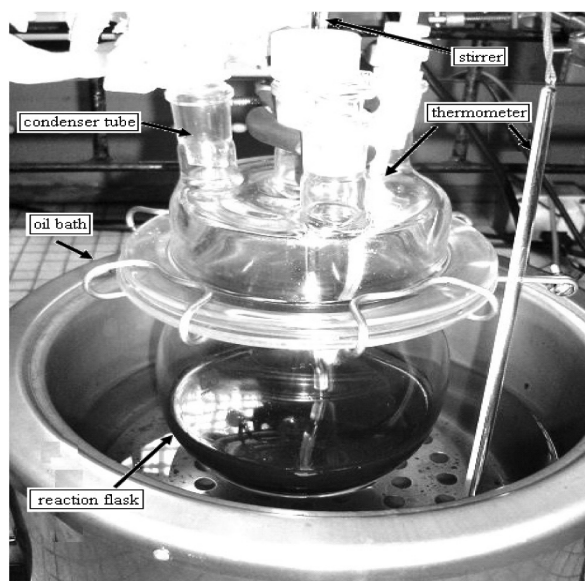
FIGURE 1. The 2 L laboratory scale synthesis reactor
